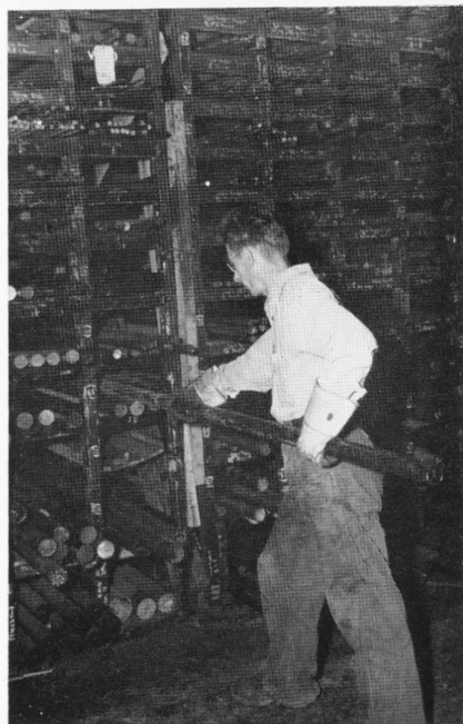
Michael Mazeika is drawing a rod from steel storage racks in Steel Stores. Note that heavier bars are located in the lower compartments.
